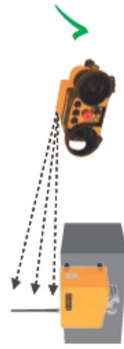
Please note when positioning the receiver unit that the antenna is free of shielding materials. If such a mounting of the receiver unit is not possible, please use an antenna extension to mount the antenna in a suitable position.
